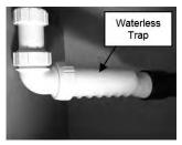
cape into the RV interior. The waterless trap can be unscrewed from the water lines. A label has been placed near the location of the waste valve that reads as follows:
