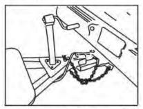
Properly mounted safety chains. Note that the jack is fully raised and dolly wheel removed.
