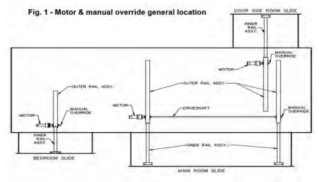
7. Locate the manual override for the slideout system (Fig. 1).
