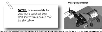
.The water pump switch should be in the OFF position when the RV is left unattended for any amount of time. If something would happen to the water system, this may help limit water damage to a smaller area.
